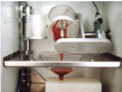
Vacuum casting process provides parts with best visual appearance and highest mechanical properties
