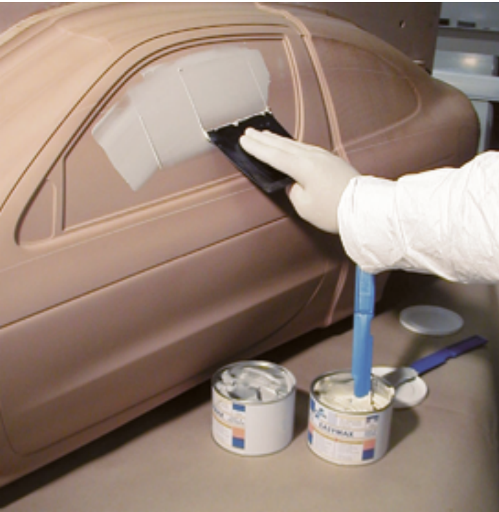
Easymax perfect match repair putty to medium density boards having the same PUR chemistry with quick setting and odour-less
