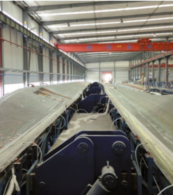
Vacuuminfusion of a wind blade with Biresin® CR131
