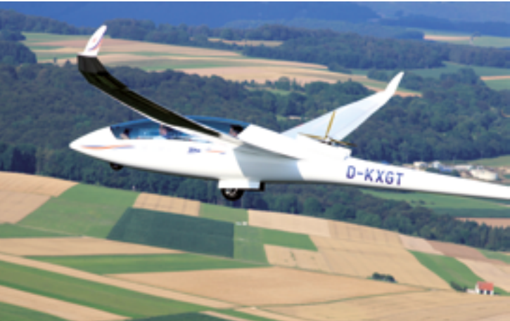
Motorglider produced by Schempp-Hirth with Biresin® CR122
