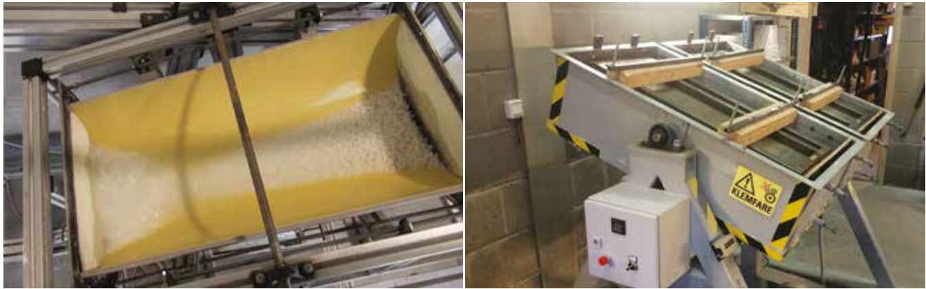
Above: Abrasion resistance test. Below: Long-term ring stiffness test.
