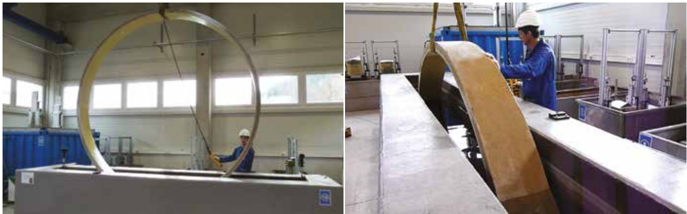
Above: Abrasion resistance test. Below: Long-term ring stiffness test.
