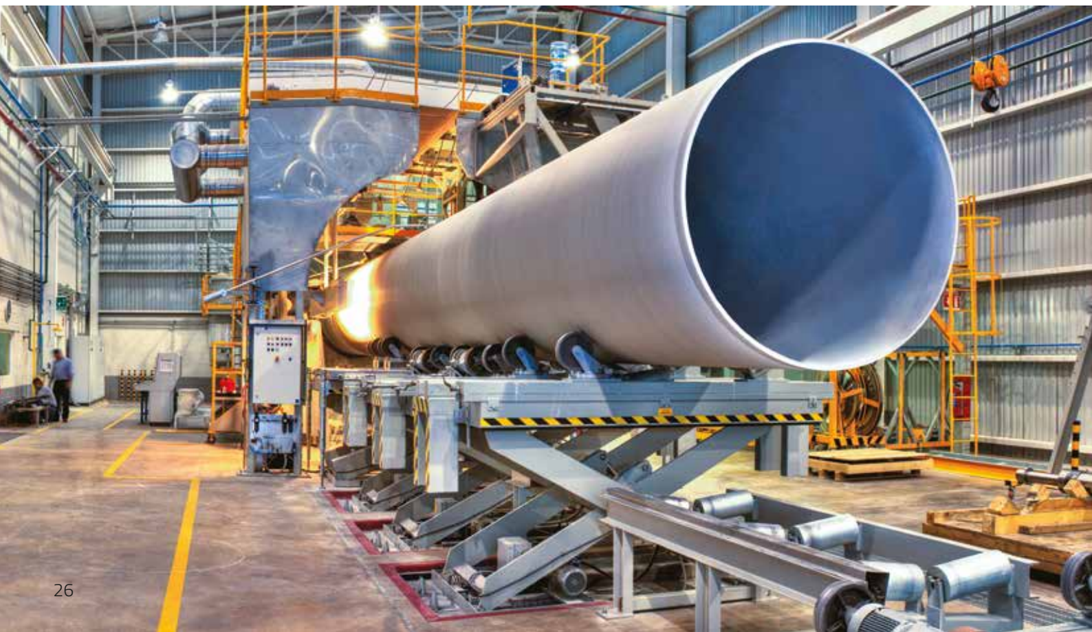
Flowtite pipe produced by continuous filament winding.
